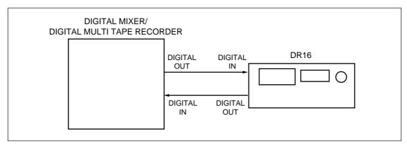
In the diagram shown above, the external digital device is set as a slave machine, and is synchronizing with the DR16's internal digital clock. However, the DR16 is also trying to lock to the external digital clock. This situation prevents synchronization. In order to avoid this, you can set the DR16 so that it will ignore the external digital clock fed from its digital input connector and reference the internal clock. (AutoSync: OFF)
